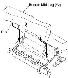
Figure 18 - Installing Bottom Mid Log
